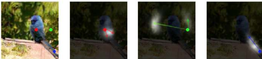
Figure 9-10. A SAGAN-generated image of a bird (leftmost cell) and the attention maps of the final attention-based generator layer for the pixels covered by the three colored dots (rightmost cells) 11
